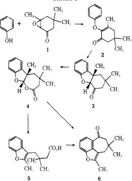
solution of lactone 4 with excess titanium tetrachloride. Partitioning the reaction components between ether and 1 N sodium hydroxide solution gives pure ketone 6 (mp 88–89 °C, 94% isolated yield) in the organic layer. Acidification of the sodium hydroxide layer gives, after ether extraction, carboxylic acid 7 in 1.4% yield.
